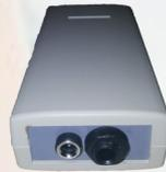
This is the basic model and is not customisable other than the connection required by your current Nurse Call system. The basic version is fitted with one(1) input socket for the bed-mat and power jack.
